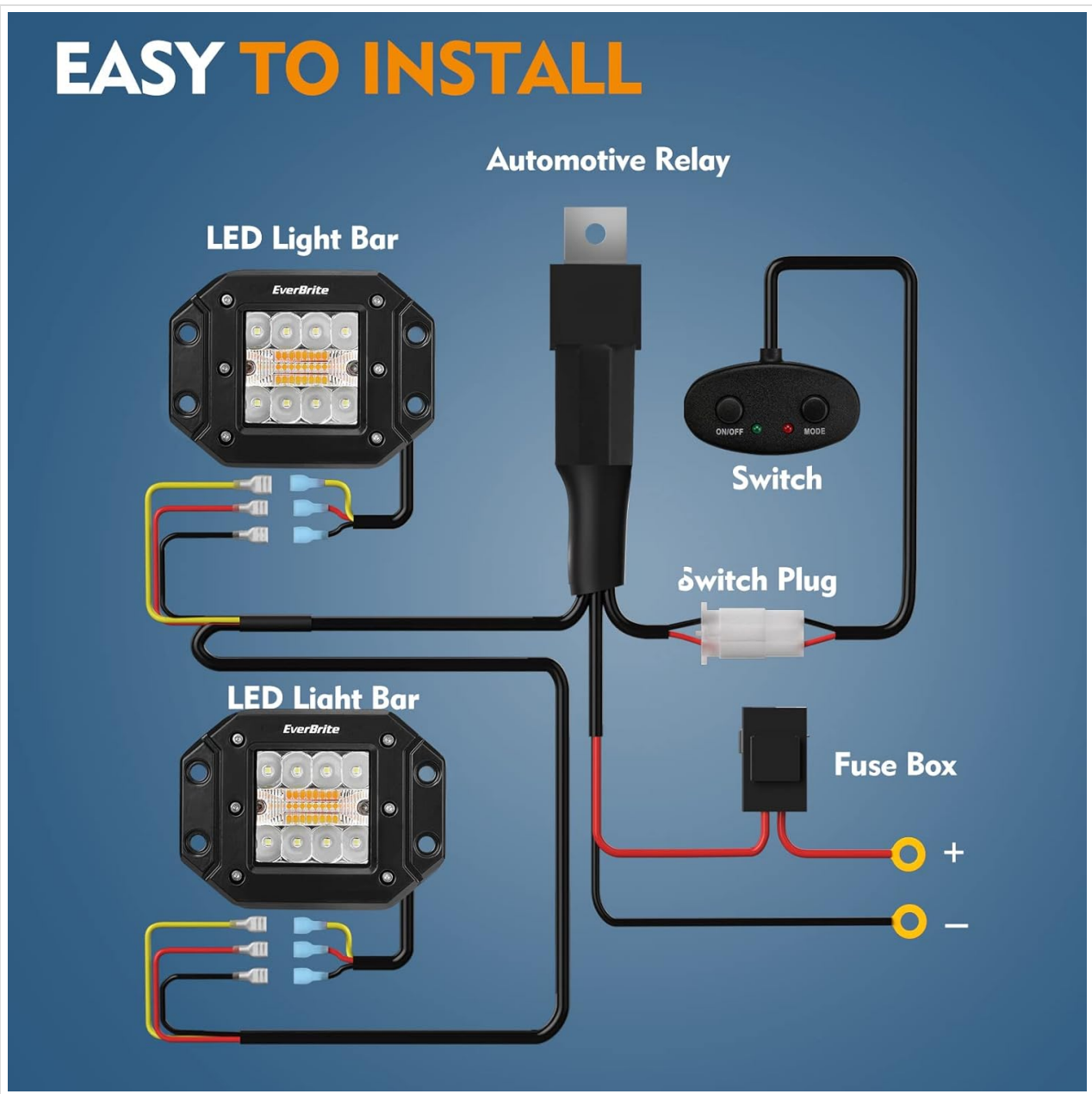
Figure 4.1: Detailed wiring diagram for connecting the EverBrite LED Light Pods to your vehicle's electrical system using the provided harness.
