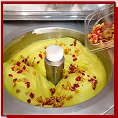
Figure 4.2: The agitator mixes the ingredients under the transparent lid. Additional ingredients can be added during this stage.
