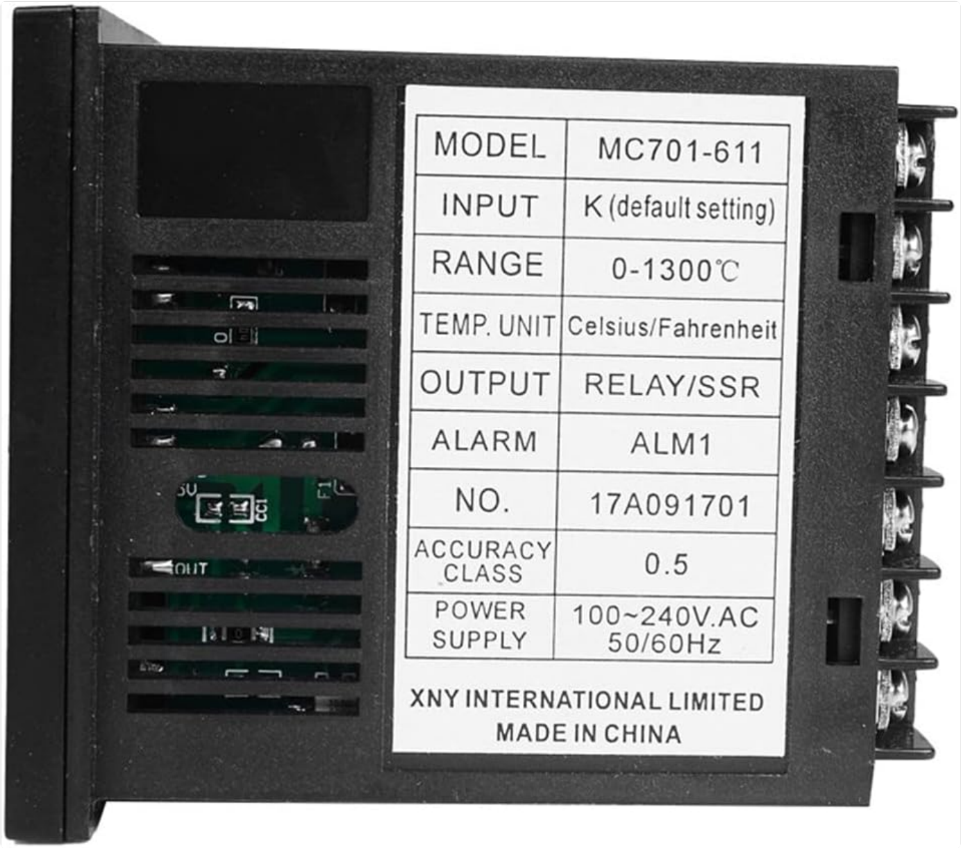
Figure 8.1: Side view of the MC701 controller displaying its detailed specification label.
