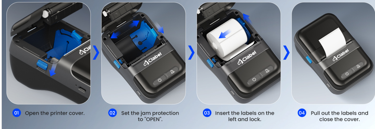
Image: Step-by-step guide for label installation, showing opening the cover, setting jam protection, inserting labels, and closing the cover.
