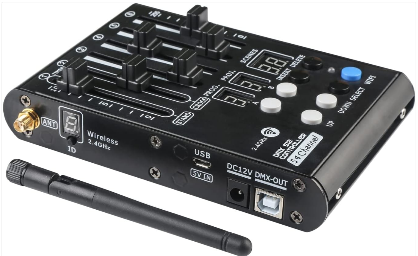
Figure 4.2: Side view of the controller, illustrating the USB 5V IN, DC 12V DMX-OUT, and USB DMX-OUT ports, along with the wireless antenna connection.
