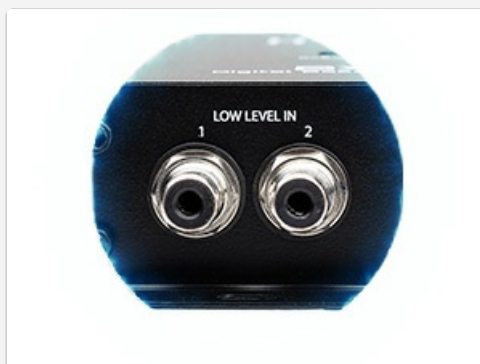
Image 2.3: Detailed view of the low-level RCA inputs on the Hifonics BXIPRO1.5.
