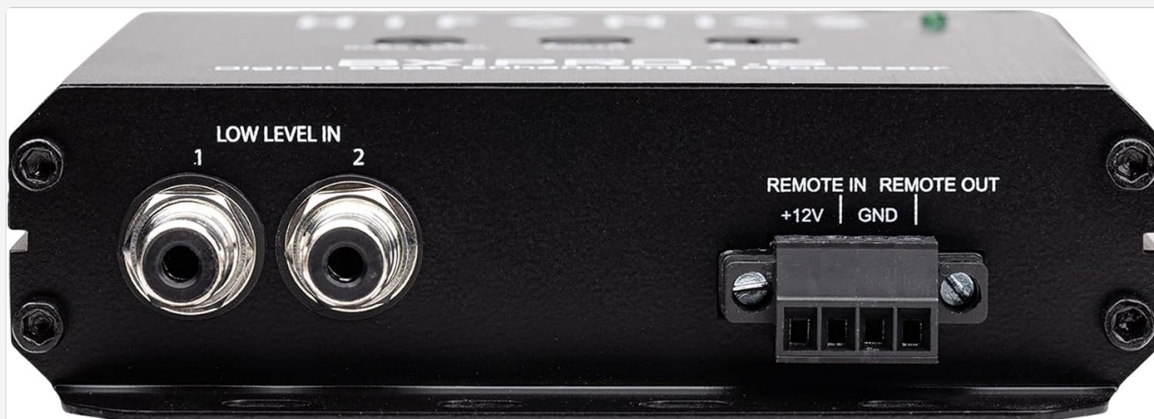
Image 2.2: Rear view of the Hifonics BXIPRO1.5, illustrating the low-level inputs (1 and 2) and the power/remote terminals (+12V, GND, REMOTE IN, REMOTE OUT).
