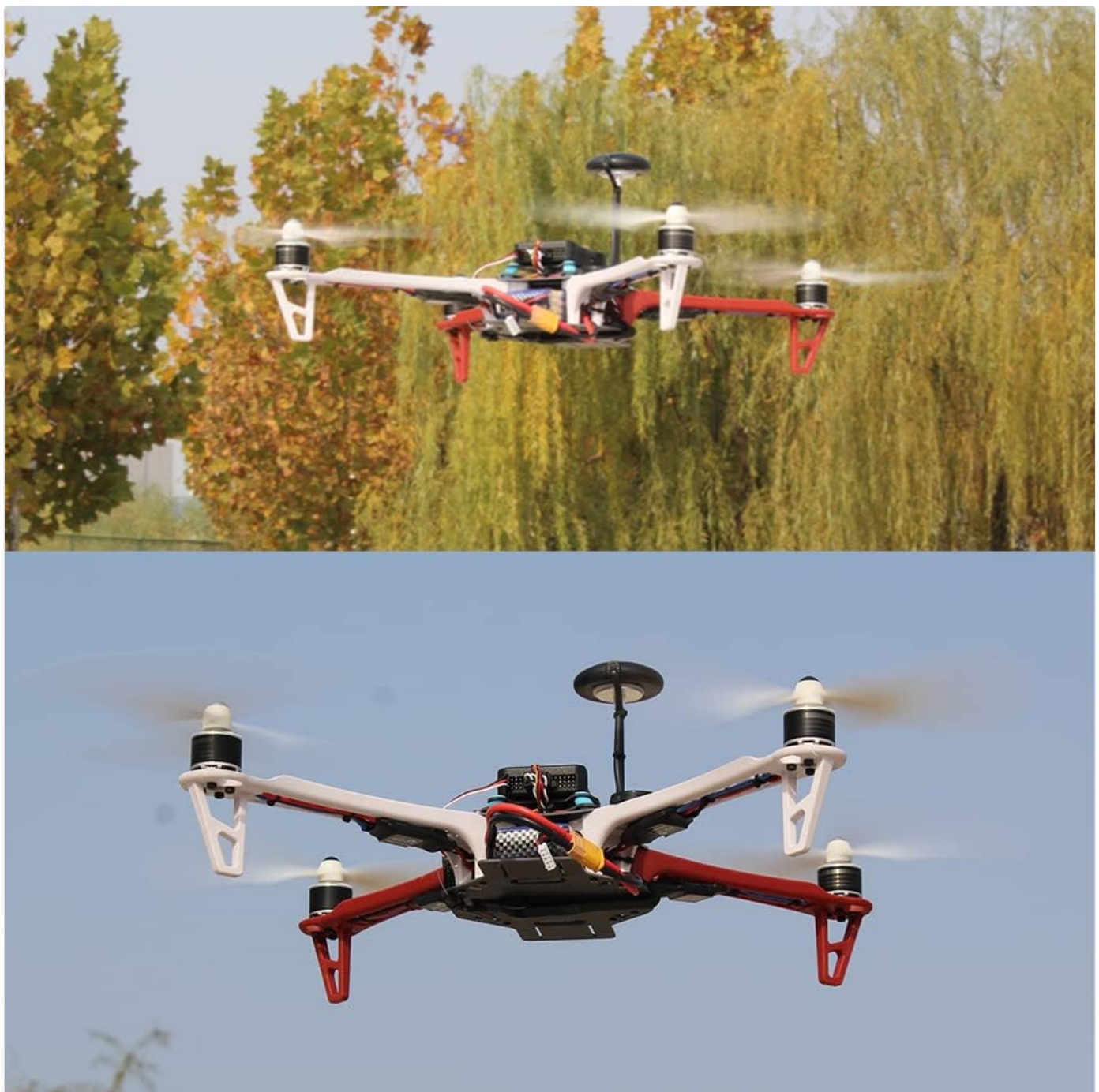
Image: Motors attached to the drone arms.
