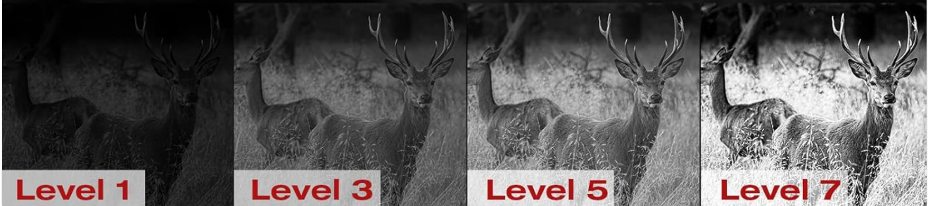
Figure 4.2: Adjustable IR levels provide optimal visibility in varying dark conditions.
