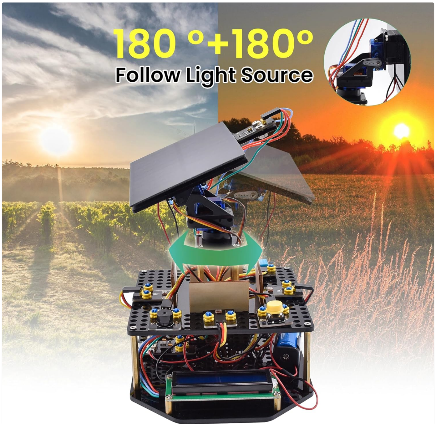
Figure 4: The solar panel automatically adjusts its position to follow the light source.
