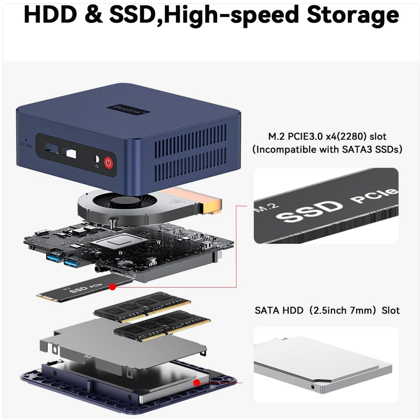
Figure 6: Internal layout highlighting the M.2 SSD and RAM slots for easy upgrades.
