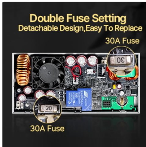
Figure 7.1: Internal view of the RD6024 showing the location of the double fuse setting for easy replacement.
