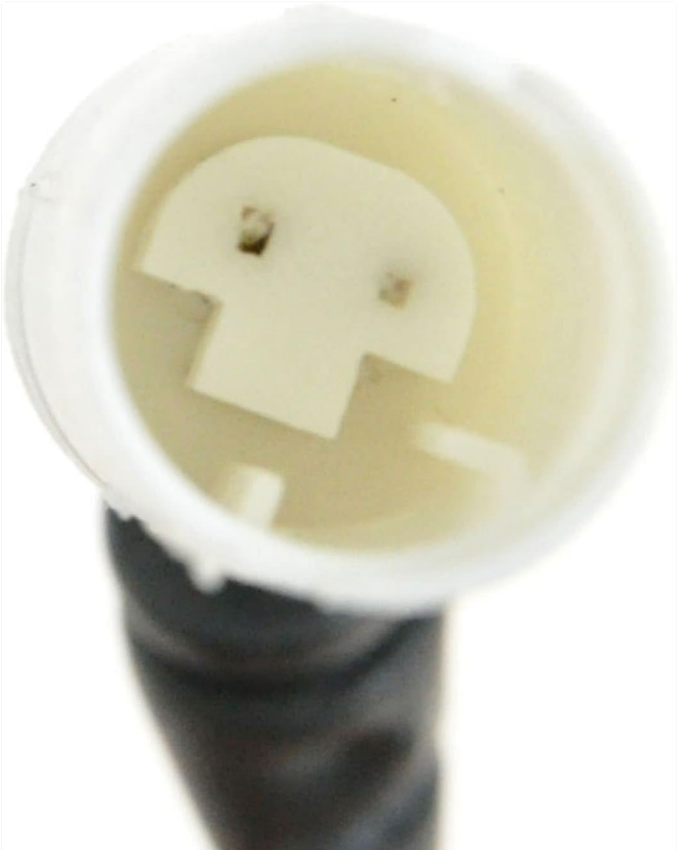
Image: A close-up view of the brake pad wear sensor, a component that indicates when brake pads need replacement.
