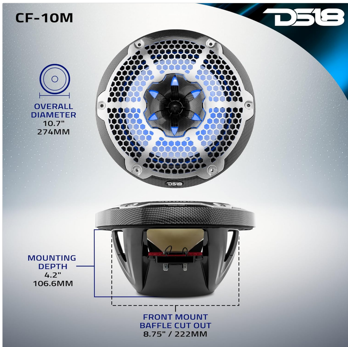
Figure 1: Speaker Dimensions for Installation
