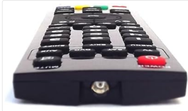
Image: This image shows the top end of the remote control, where the infrared (IR) emitter is located. This part should be pointed towards the device being controlled.
