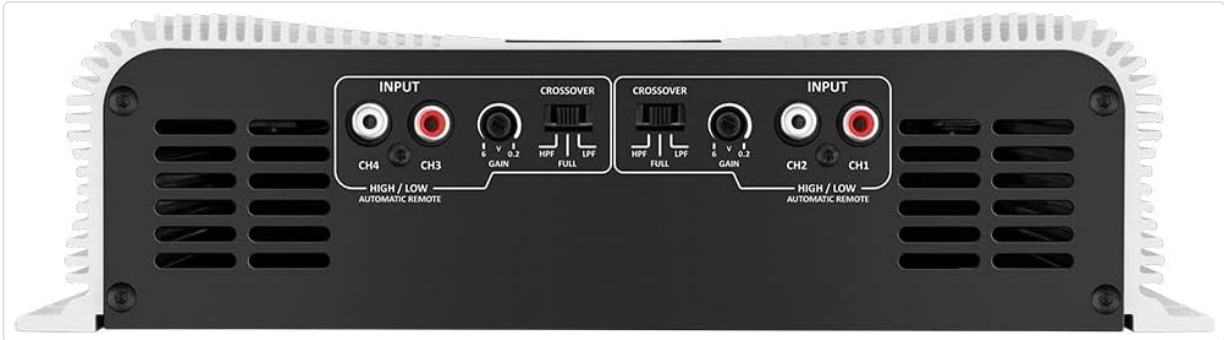
Figure 3.2: Rear view of the amplifier showing RCA inputs, gain controls, and crossover switches for channels 1-4.
