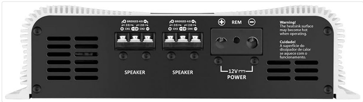
Figure 3.3: Rear view of the amplifier showing power input terminals and speaker output terminals.
