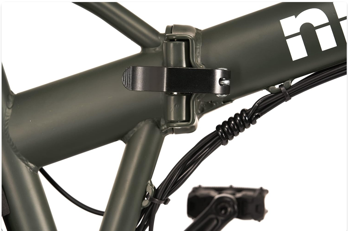
Image 4.1: Detail of the frame's folding hinge and quick-release lever.
