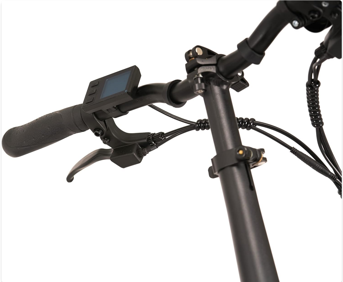
Image 5.1: The LCD digital display, providing ride information.
