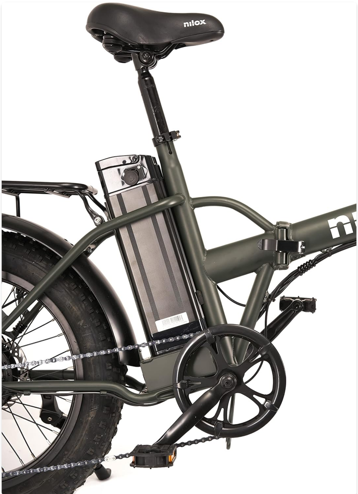
Image 4.3: The removable lithium-ion battery pack, located on the frame.
