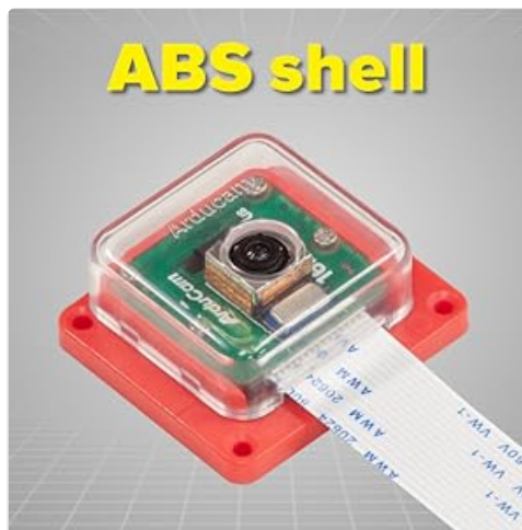
Image 3.3: The camera module housed within its protective ABS shell.
