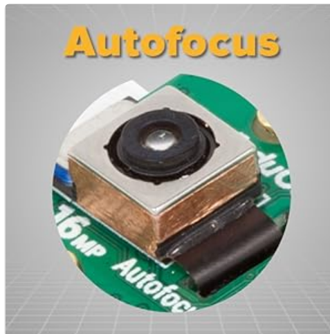
Image 3.2: Close-up of the autofocus lens mechanism.
