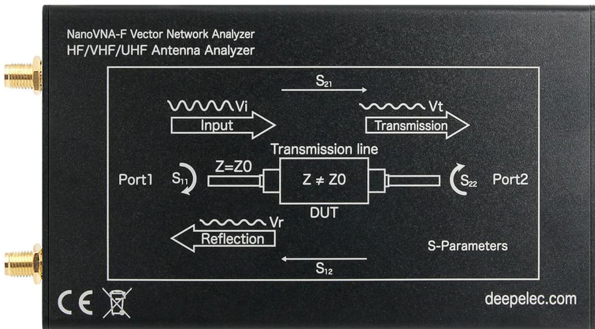
Figure 3: Schematic representation of S-parameter measurement connections on the NanoVNA-F V3.1.
