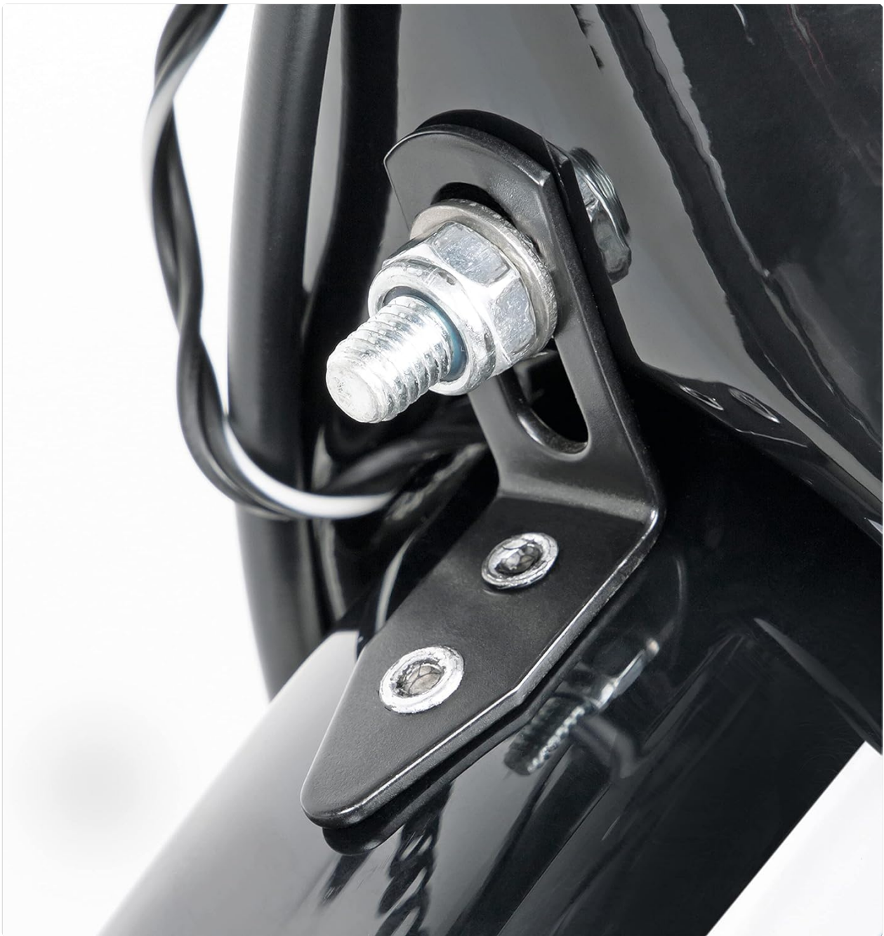
Figure 4: Front fender mounting bracket secured to the bicycle fork, illustrating the attachment method.
