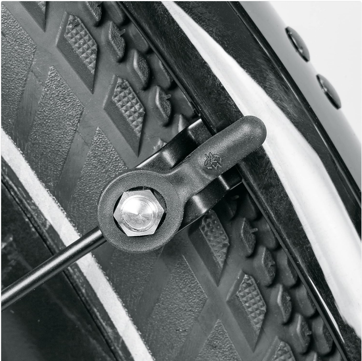
Figure 3: Detail of a fender stay attachment point, showing the bolt and nut assembly.
