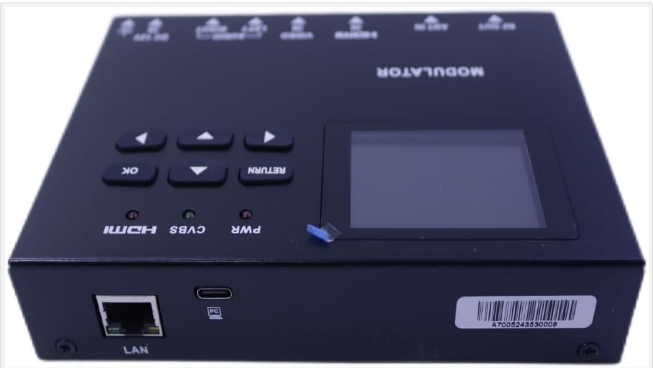
Figure 2.2: Detailed front view of the modulator, showing the RF OUT, ANT IN, HDMI IN, VIDEO IN (RCA), AUDIO IN (Left/Right RCA), and DC 12V IN ports.
