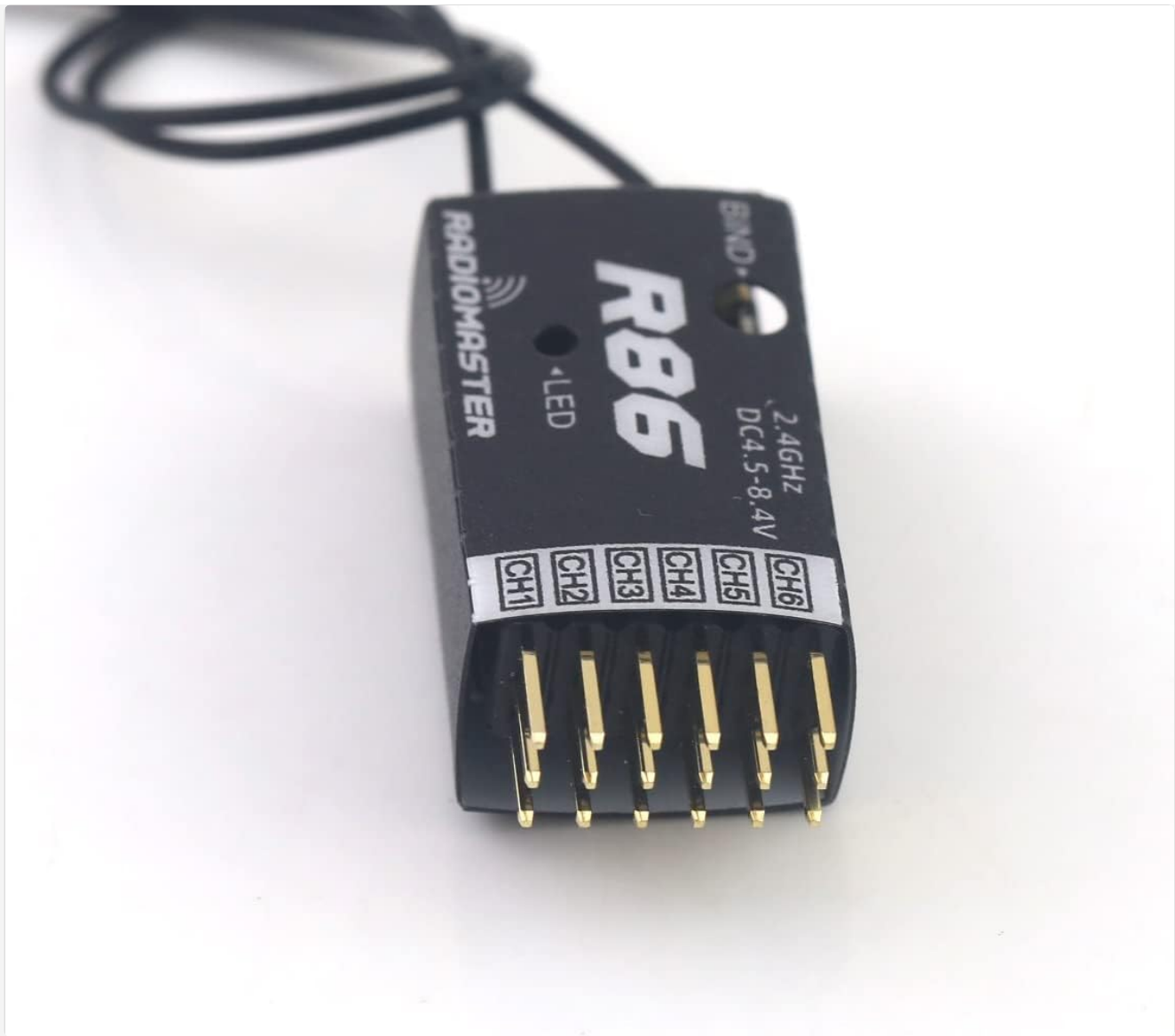
Image 2.2: Close-up view of the R86 receiver's pin headers, labeled CH1 through CH6, for PWM and SBUS connections.
