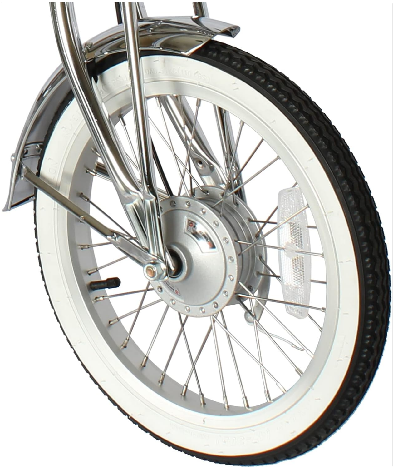
Image 2.1: Detail of the front wheel and drum brake assembly.
