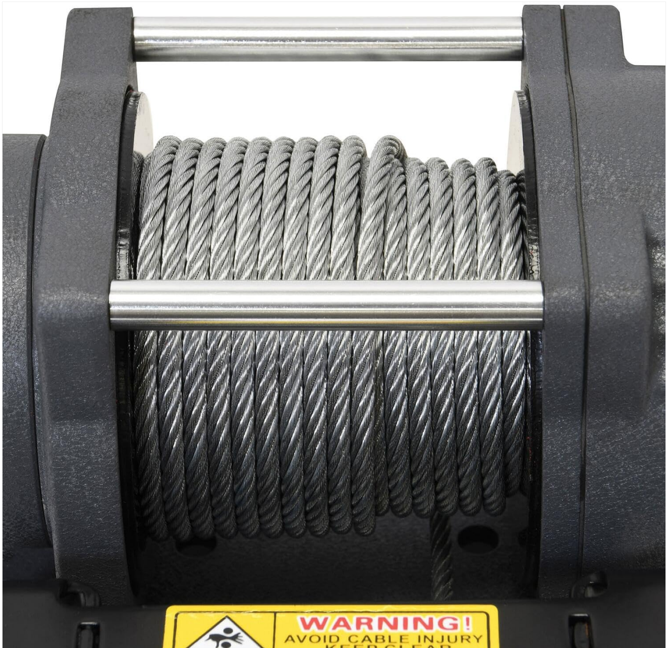
Image 6.1: A close-up view of the steel rope properly spooled on the winch drum, highlighting the importance of regular inspection.
