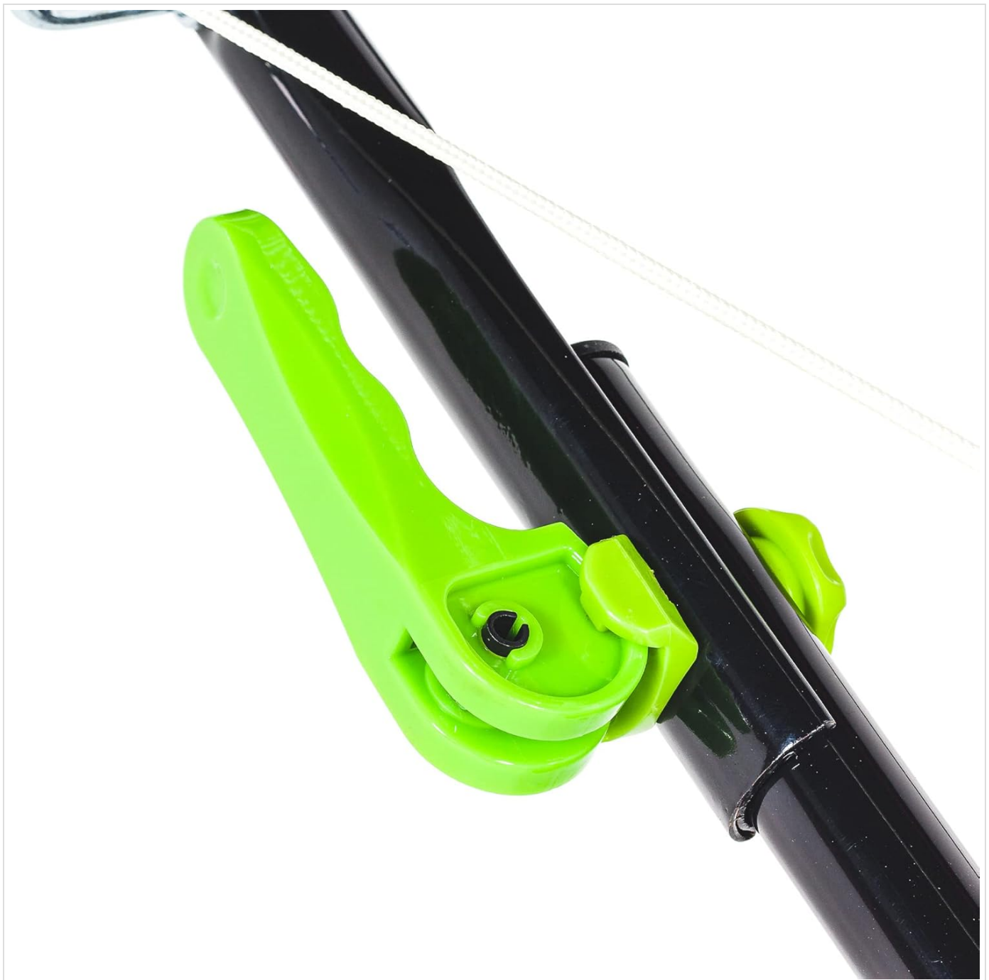
Figure 7: Handlebar control lever. This image shows the green lever on the handlebar, which is typically the operator presence control bar that must be held to allow the engine to run.
