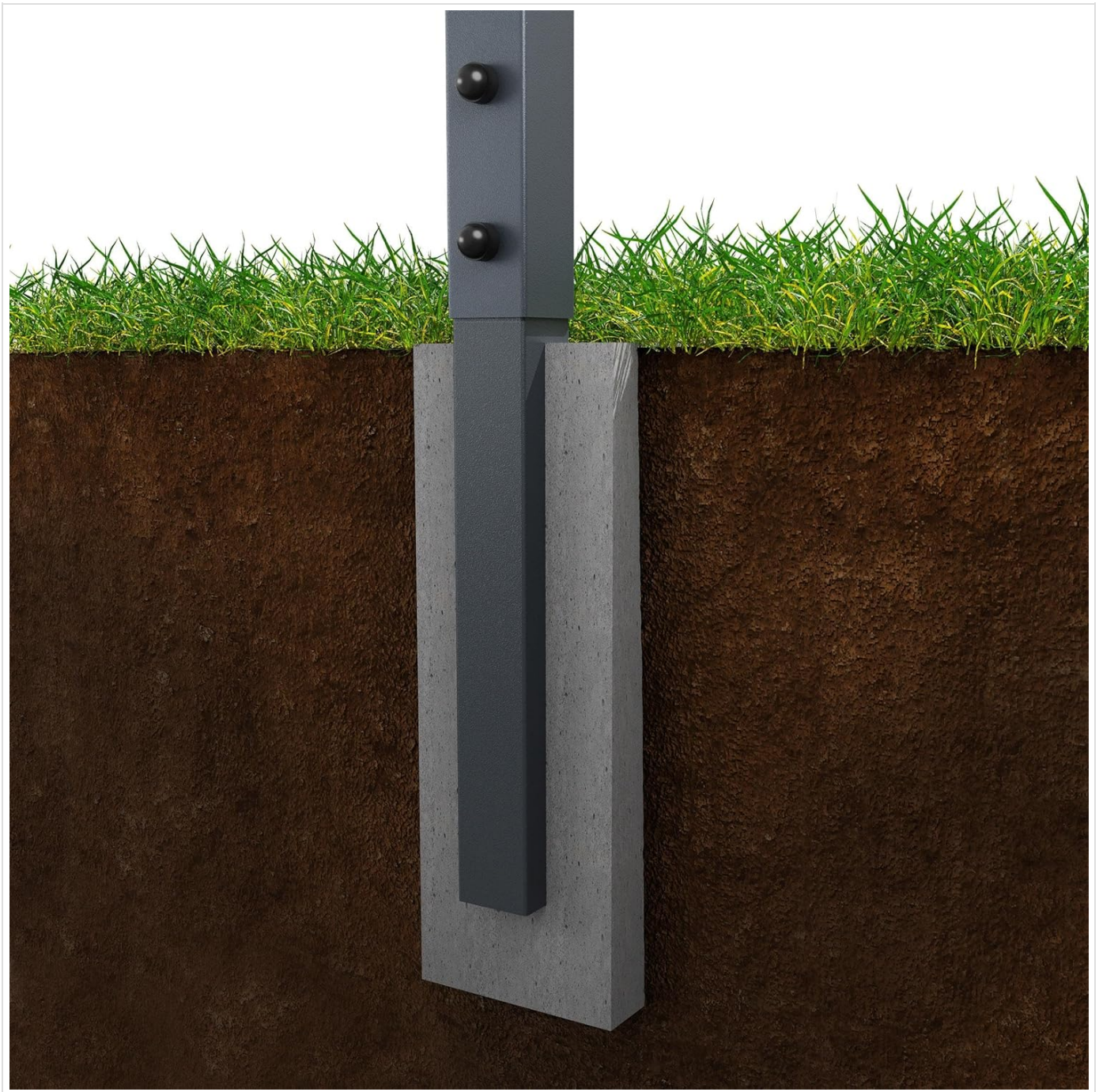
Figure 3.1: Illustration of secure ground anchoring. This image depicts how the main support posts of the calisthenics bar are to be embedded into the ground, showing the required depth and the use of concrete for maximum stability.
