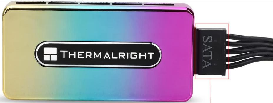
SATA direct power input, continuous and stable output under overload conditions
