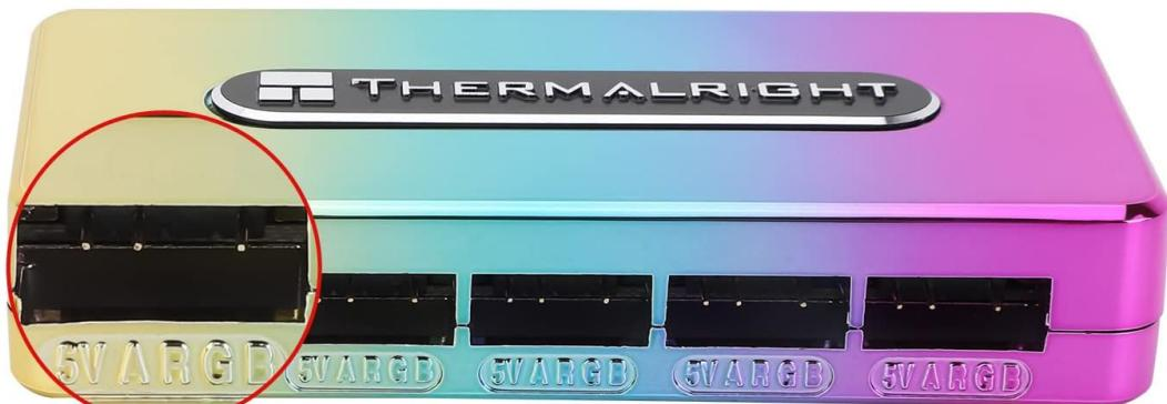
Supports 3pin+5V interface devices such as ARGB fans, ARGB light strips and other similar devices
