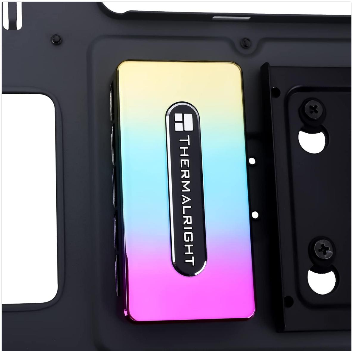
*Image: The ARGB hub securely mounted to the back panel of a PC case using its double-sided adhesive tape.*
