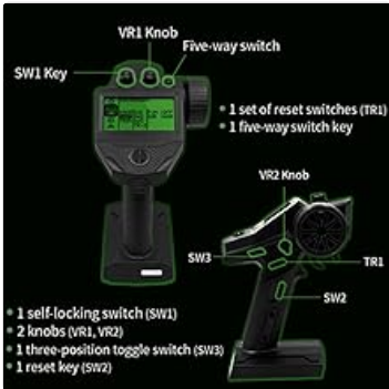
Image 5.1: Diagram illustrating the reasonable layout of controls on the FS-G7P transmitter, including knobs, switches, and the five-way switch for menu navigation.
