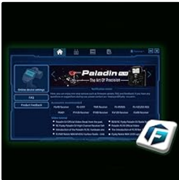
Image 6.1: Screenshot of the FlySky Assistant 3.0 software interface, used for firmware upgrades, model data storage, and copying.
