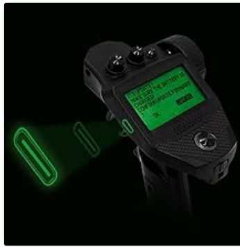
Image 2.3: Depiction of the Type-C data port on the FS-G7P, indicating its use for firmware upgrades, external power, and simulator connections.
