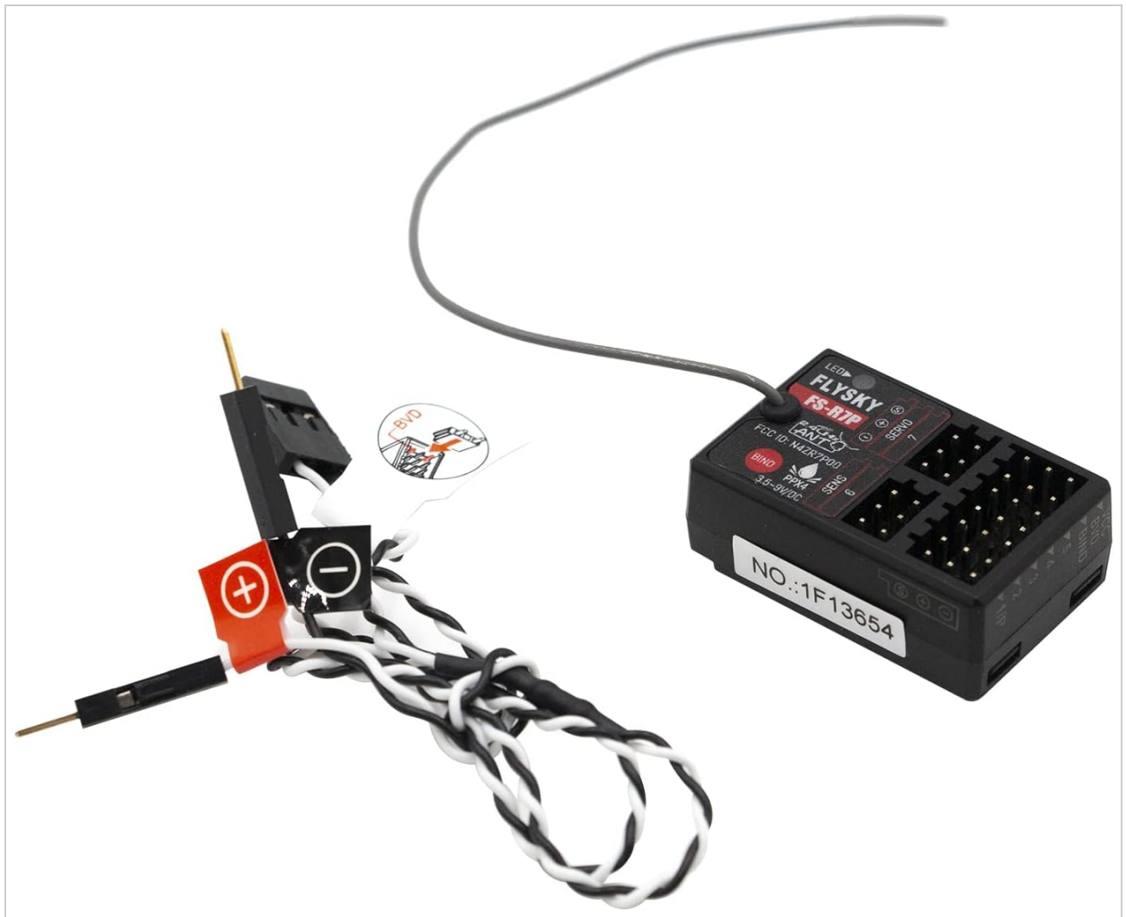
Image 5: The FS-R7P receiver shown with a binding plug inserted into the BIND port.
