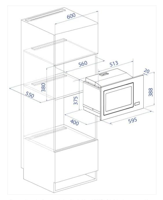
This diagram illustrates the precise dimensions for installing the Mayer MMWG25B built-in microwave oven. Key measurements include a width of 595mm, height of 388mm, and depth of 513mm, with specific cabinet cutout requirements for proper fit.
