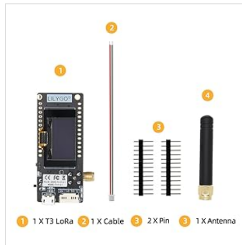
Figure 3.1: Included components with the LILYGO LoRa32 Development Board.
