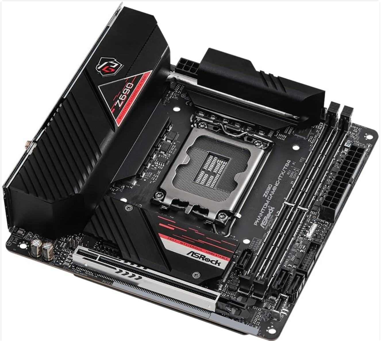
Image: Angled view of the ASRock Z690 Phantom Gaming-ITX/TB4 motherboard, showing the M.2 slots and heatsinks.
