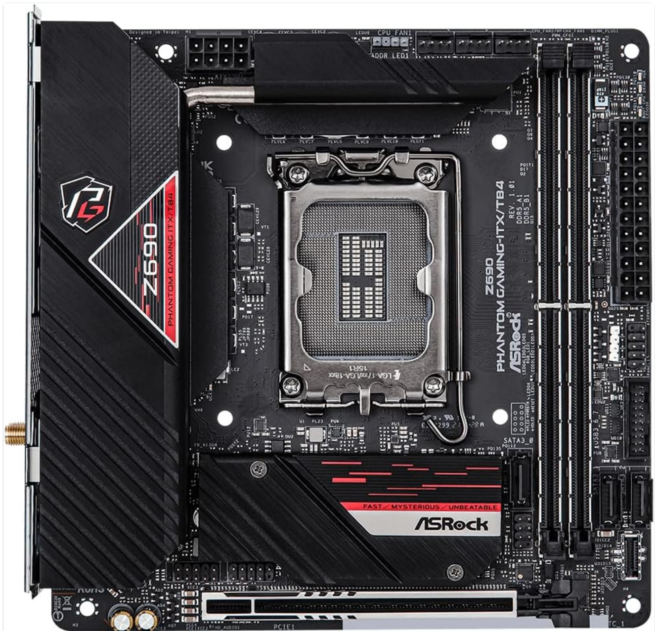
Image: Top-down view of the ASRock Z690 Phantom Gaming-ITX/TB4 motherboard, highlighting the LGA 1700 CPU socket.
