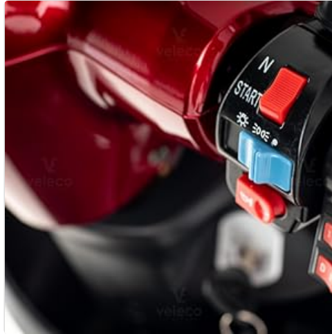
Figure 5.1: Handlebar controls including the 'START' button and speed selector.
