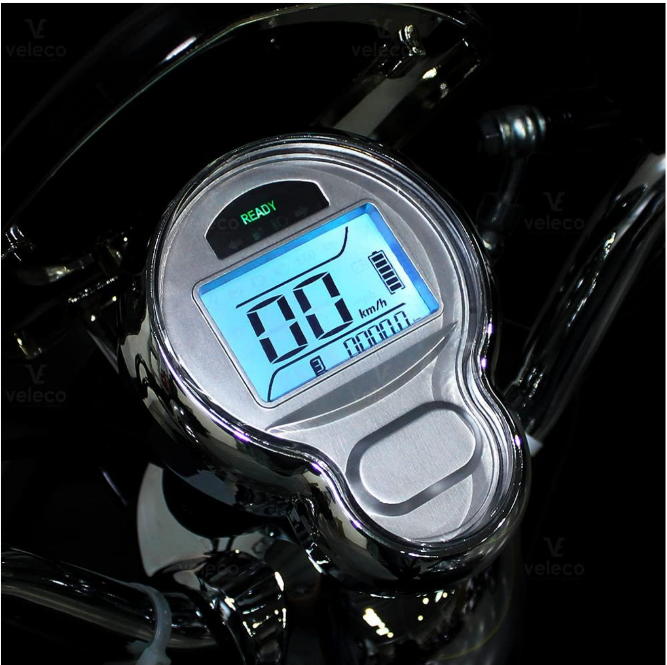
Figure 5.1: Dashboard display showing speed, battery level, and readiness indicator.
