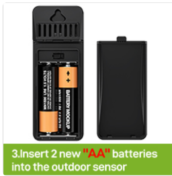
Image: Illustration of inserting AA batteries into the outdoor sensor.
