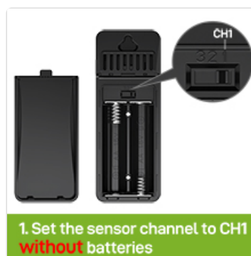
Image: Close-up of the outdoor sensor showing the channel switch set to CH1.
