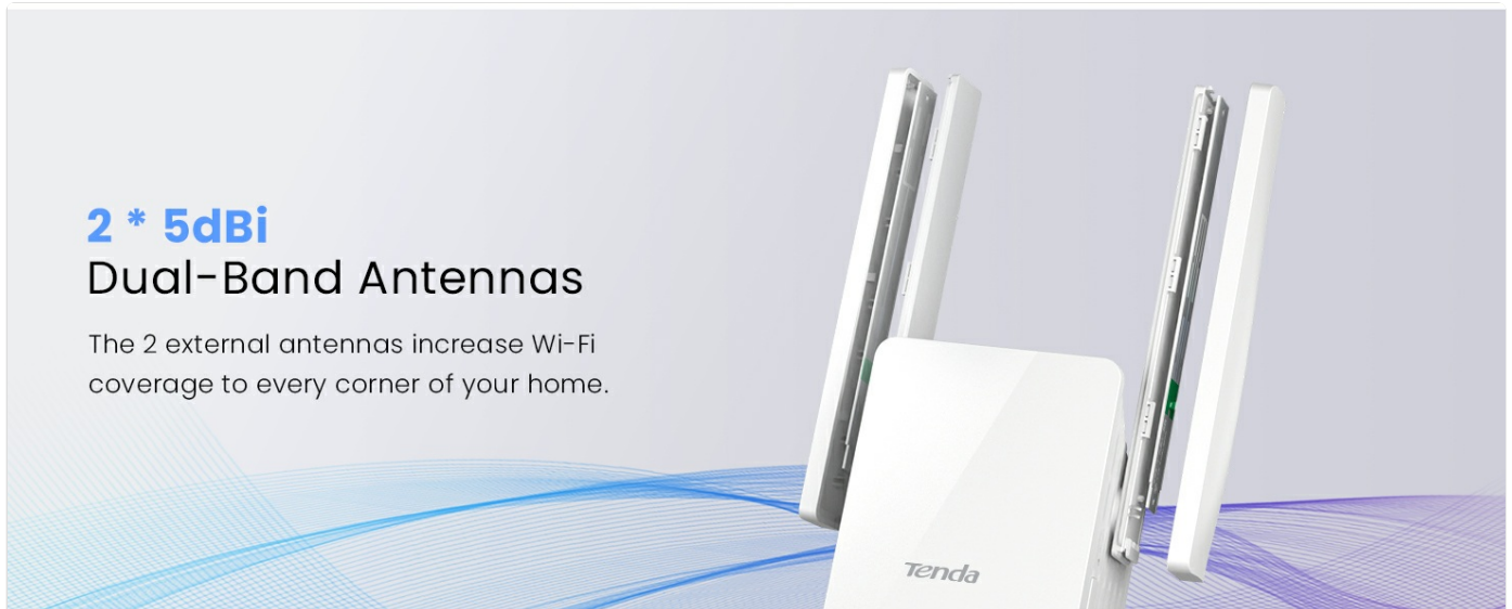
Image: Close-up of the Tenda A27 highlighting its two 5dBi dual-band antennas.
