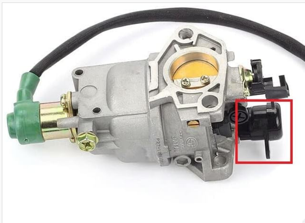
Figure 4.3: Detail of the auto choke solenoid connection. Ensure electrical wires are securely attached.
