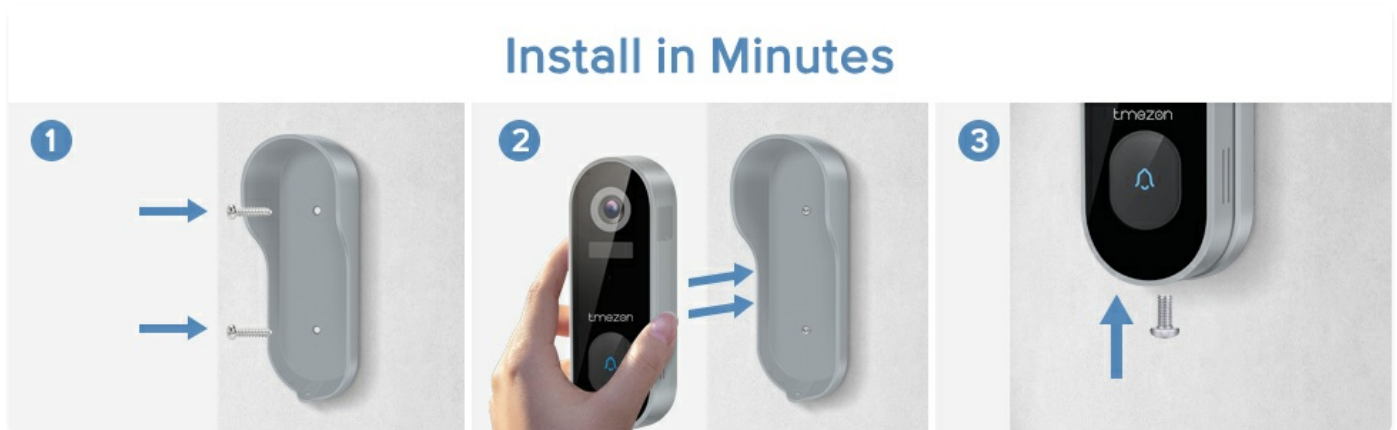
Image: Three-step illustration showing how to install the TMEZON doorbell: 1. Screw the mounting plate to the wall. 2. Slide the doorbell onto the plate. 3. Secure with a bottom screw.
