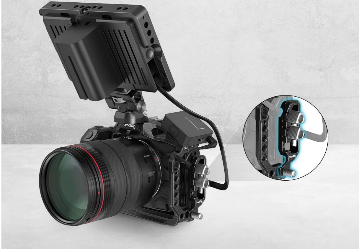
Figure 5: Multiple mounting options available on the half cage, including 1/4"-20 threaded holes, 3/8"-16 locating holes for ARRI, cold shoe, and a built-in Arca-Swiss plate.
