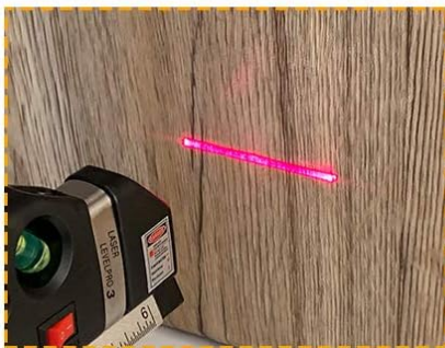
Image 5.2: The laser level demonstrating its three projection modes: horizontal line, vertical line, and cross line, useful for various alignment tasks.
