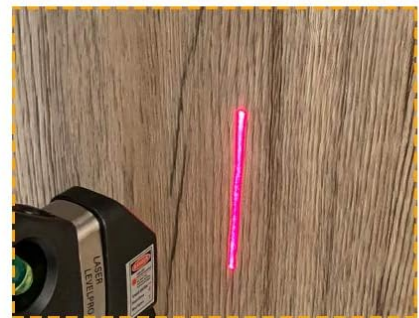
Image 5.2: The laser level demonstrating its three projection modes: horizontal line, vertical line, and cross line, useful for various alignment tasks.
