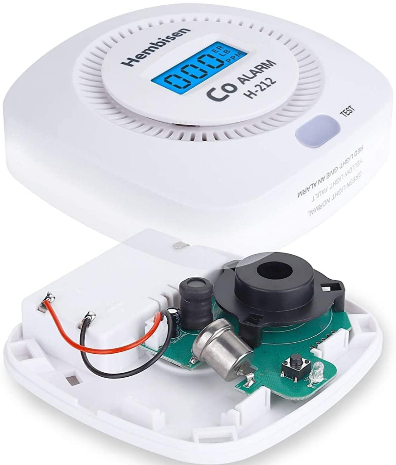
Figure 2.3: Internal view highlighting the high-precision electrochemical CO sensor, designed for reliable and rapid response.
