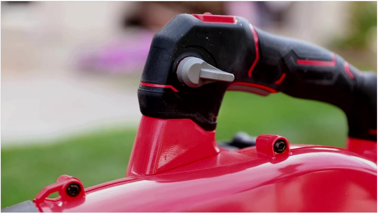
Image: Close-up of the CRAFTSMAN B2000 handle, illustrating the throttle trigger and cruise control mechanism for speed adjustment.
