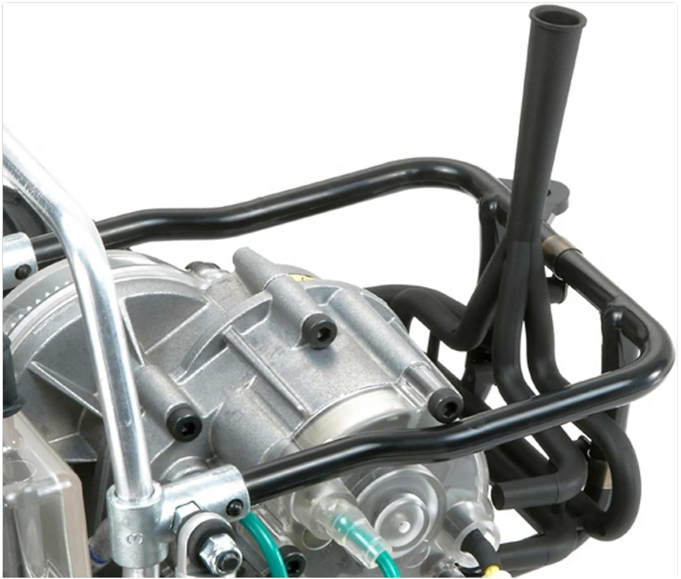
Figure 4.9: Close-up of the engine compartment and exhaust details of the TAMIYA Sand Scorcher 2010.
