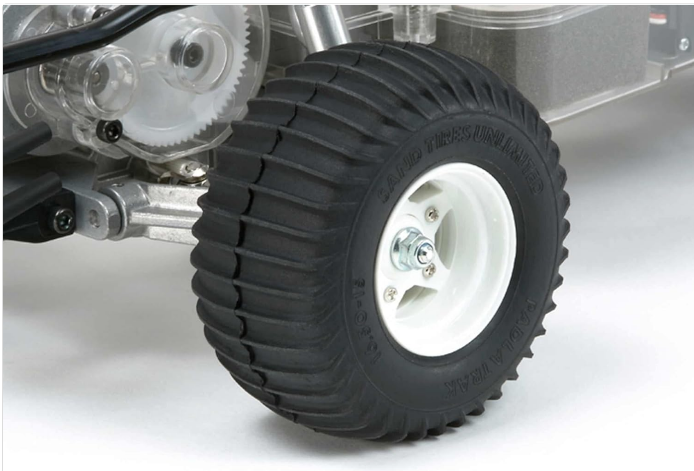
Figure 4.2: Close-up of the rear wheel featuring the unique ribbed tire design, optimized for off-road traction.
