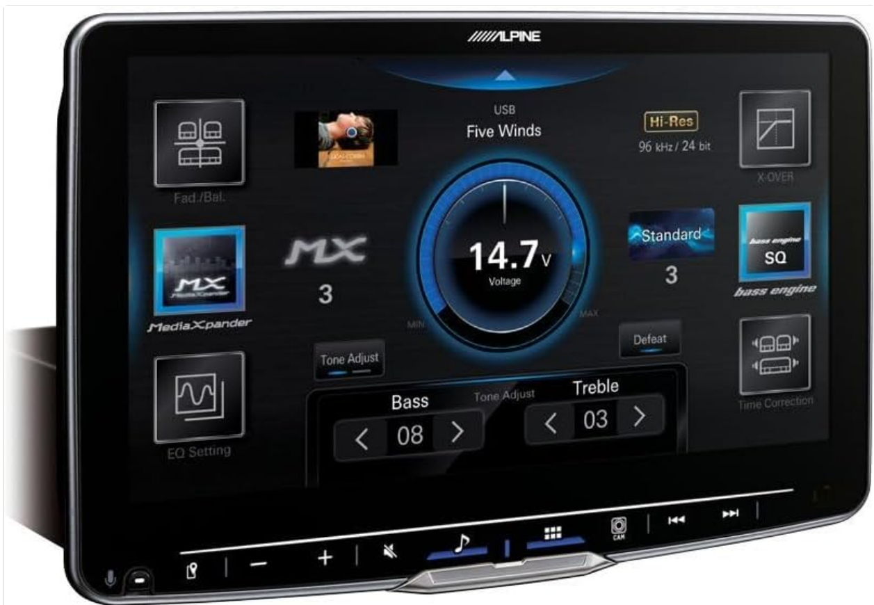
Image: The audio settings interface of the Alpine iLX-F905D, displaying options for voltage monitoring, bass and treble adjustments, and various sound enhancement features like MediaXpander and Sound Quality settings.
