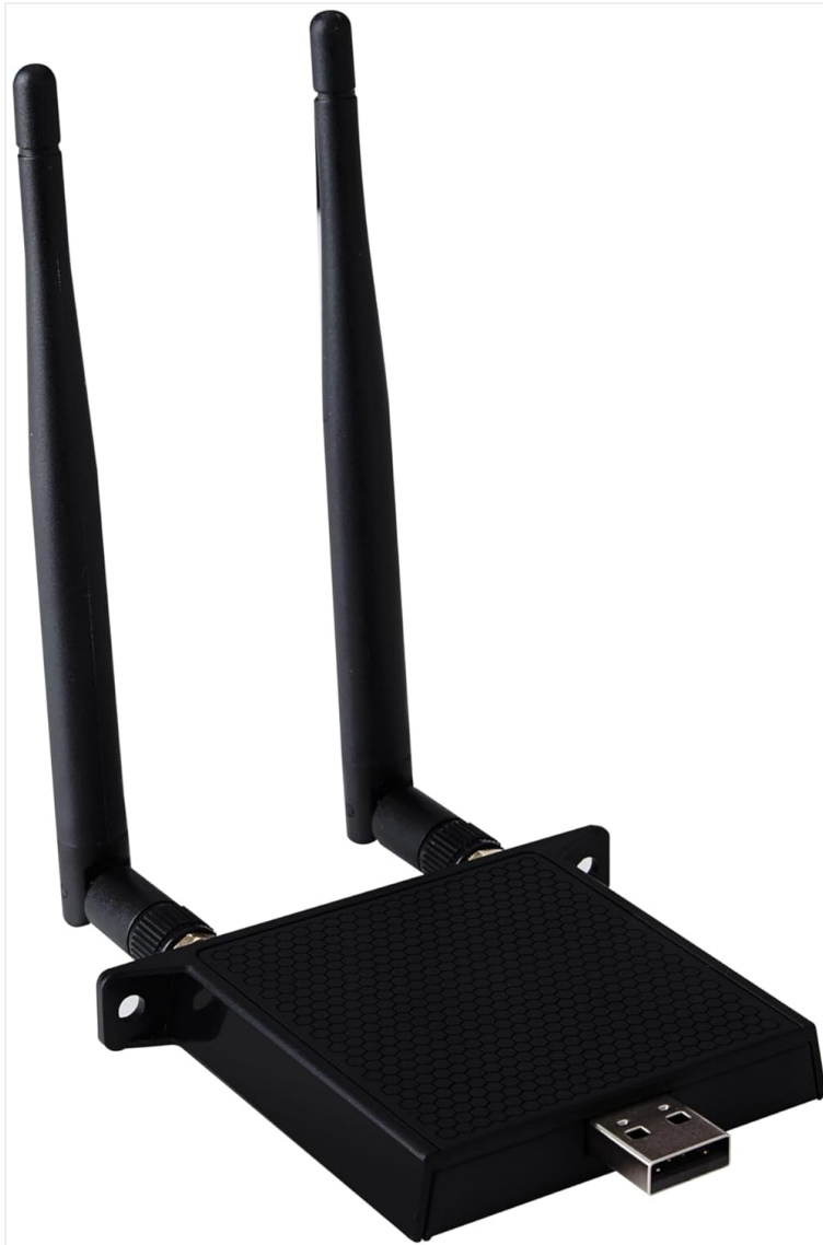
Figure 1: ViewSonic VB-WIFI-001 Dual Band WiFi 6 USB Adapter. This image shows the compact black adapter with two adjustable antennas and a USB connector.
