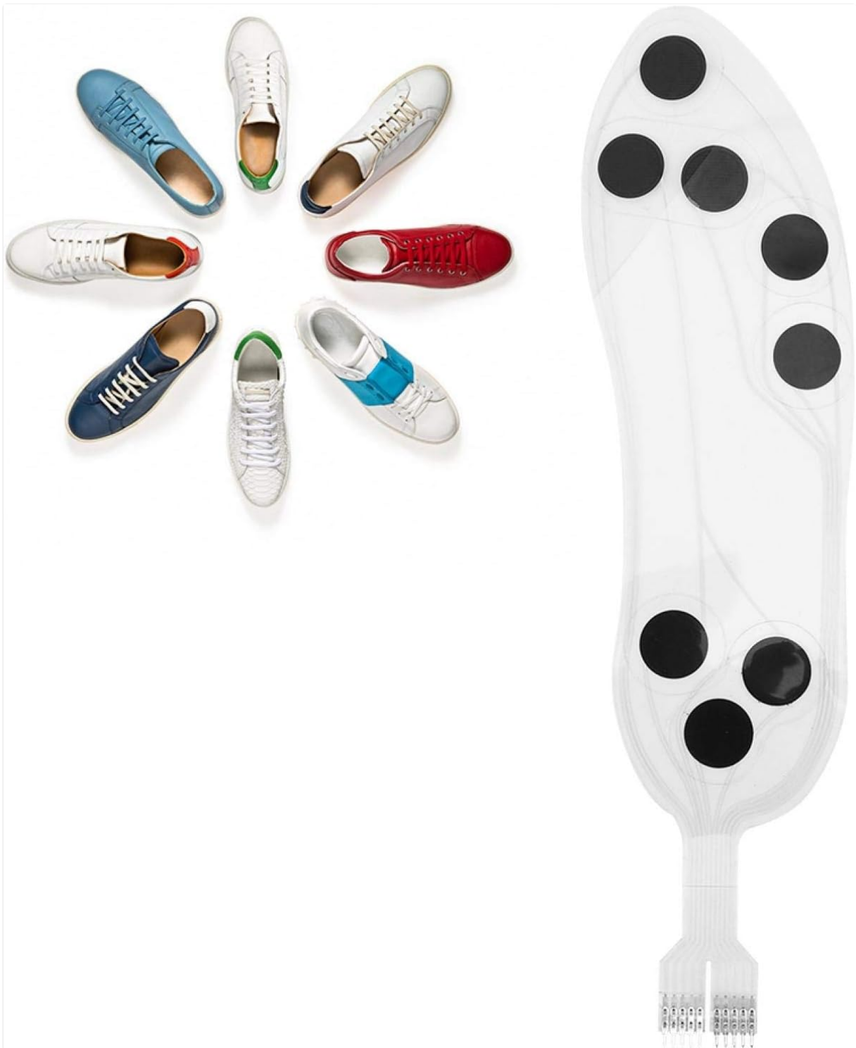
Figure 2.2: The flexible thin film pressure sensor displayed with a selection of footwear, highlighting its adaptability for use with different shoe types.
