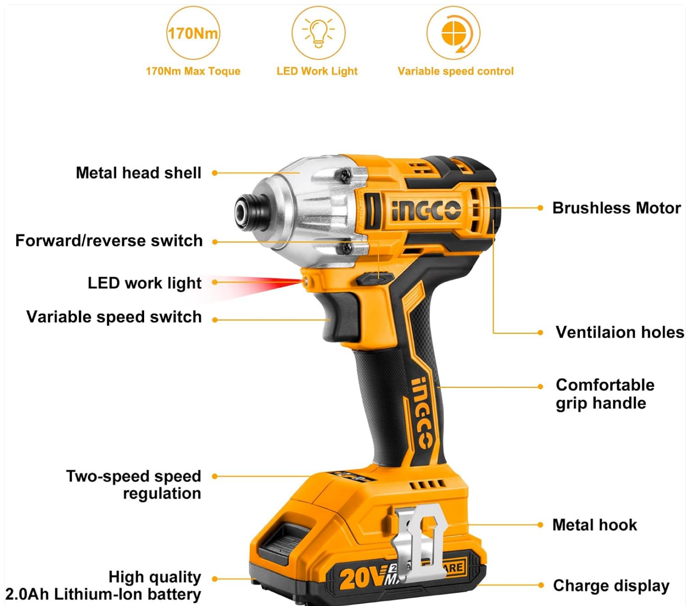
Figure 2.1: Labeled components of the Ingco 20V Brushless Impact Driver.
