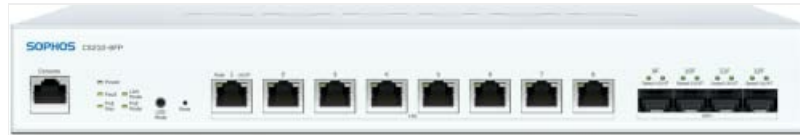
Image 4.1: Front view of the Sophos CS210-8FP Switch, showing the console port, LED indicators, eight 2.5G Ethernet ports, and four SFP+ ports.
