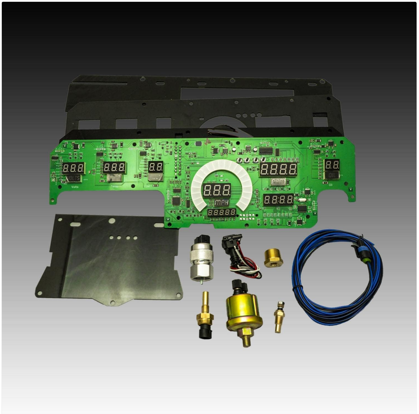
Figure 2: Included components of the gauge panel kit.
