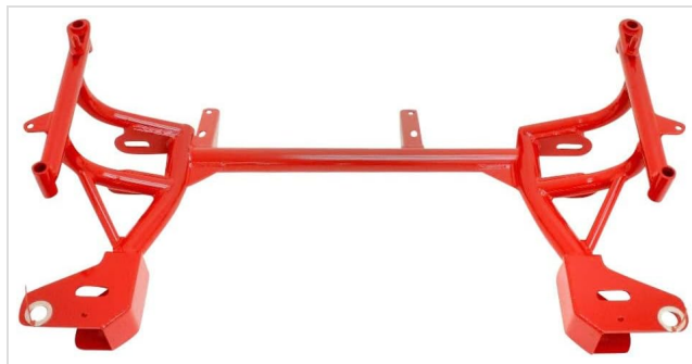
Image 1: BMR Suspension KM014-1R K-member. This image displays the red powder-coated tubular steel K-member, featuring mounting points for suspension components and a Pinto-style steering rack. The design is open for turbocharger downpipe clearance.
