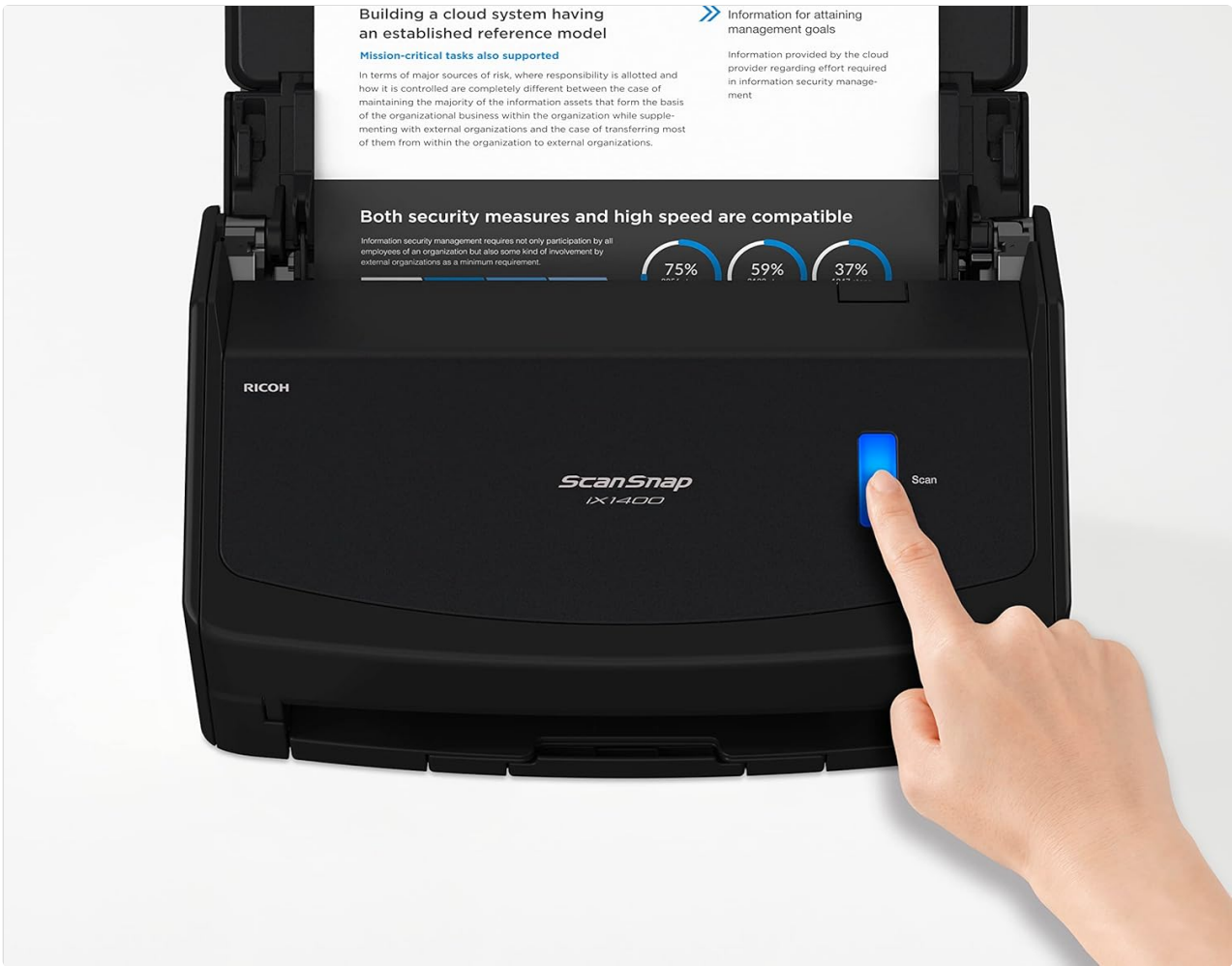
Image: The ScanSnap iX1400 with a business card and a standard document loaded in the automatic document feeder, ready for scanning.
